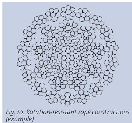
Fig. 10: Rotation-resistant rope constructions (example)
