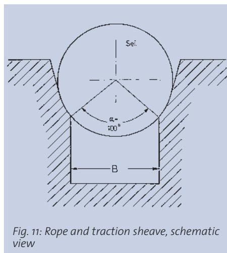
Fig. 11: Rope and traction sheave, schematic view
