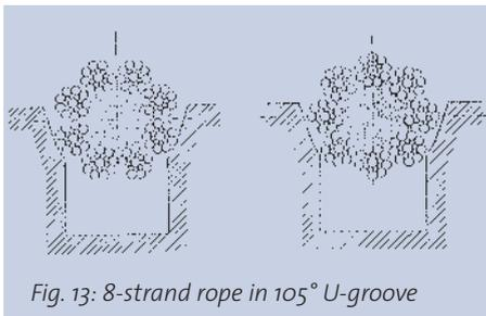
Fig. 13: 8-strand rope in 105° U-groove
