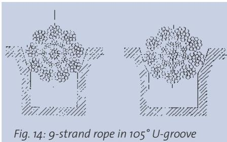
Fig. 14: 9-strand rope in 105° U-groove
