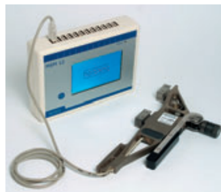
Fig. 2: Mobile rope load measuring system MSM12 and rope load sensor LSM1 from the WeightWatcher measurement system
