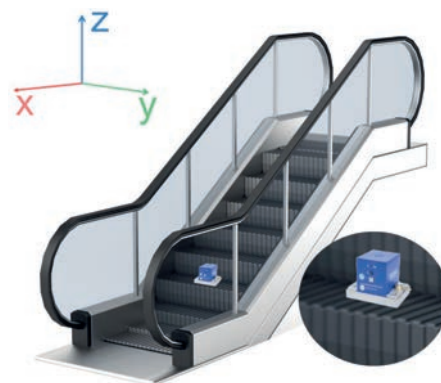
Alignment and positioning of the vibration sensor on the escalator
