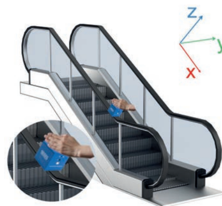
Alignment and positioning of the vibration sensor on the handrails
